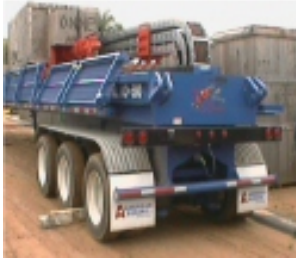
HDD Rig 1 American Augers DD 580 Mud Cleaning System 300 ton Pull Back Capacity HDD Rig Year of Purchase 2003
