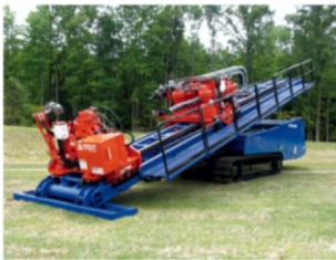
HDD Rig 3 American Augers DD 440T HDD Rig & MPR Drilling Fluid Mixing, Pumping & Recycling System mud Cleaning System Year Purchase 2008
