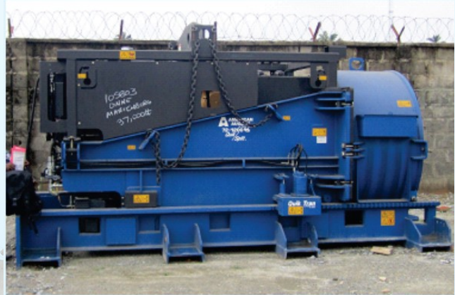
AMERICAN AUGER 72 - 1200NG HORIZONTAL EARTH BORING MACHINE - YEAR OF PURCHASE 2013
