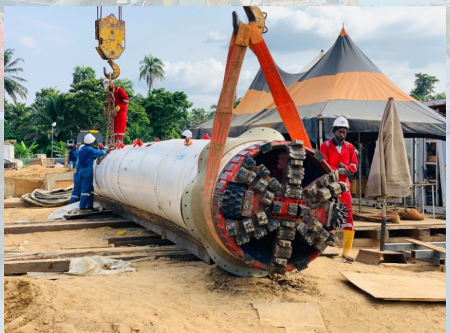
PIPE JACKING UNIT AND ACCESSORIES (800ton Push Force) YEAR OF PURCHASE 2022
